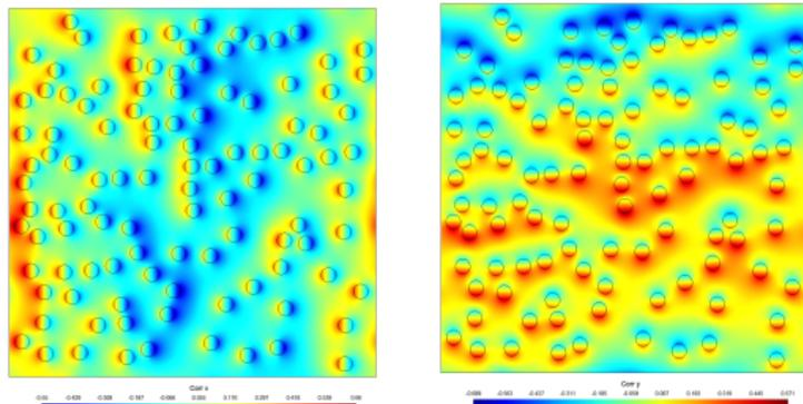
Figure: Numerical simulations of the correctors (left:  $\phi_1$ , right:  $\phi_2$ )
